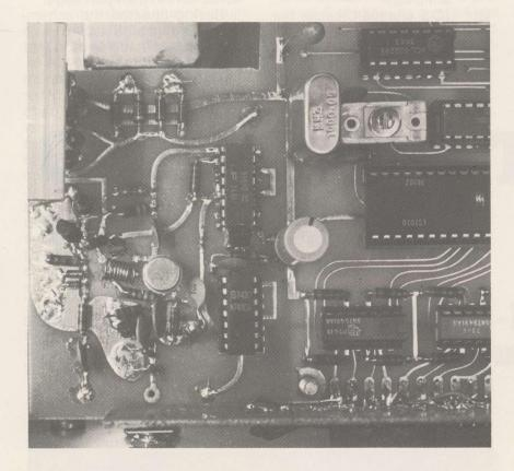
long enough to flow-solder) connect up the 95H90. Now put the board into the case (see photos) and connect the input "F" fitting and the 2 pole, 3 position switch. Note: Use very short leads (as short as practical) in wiring up the switch and the input fitting.
